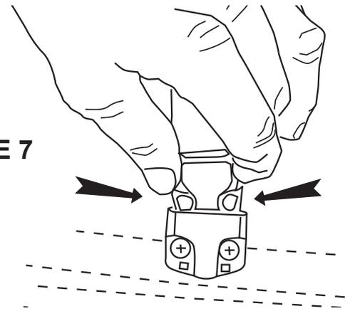
7. Verify both buckles are attached by pulling on the strap. **WARNING:** Damage to personal property and possible injury may occur, if; vehicle is operated without both retaining straps fastened securely when cover is in open position, or if the attachment clamps are not firmly secured to the box lip, or if the clamps are not properly stowed using the retention feature.
