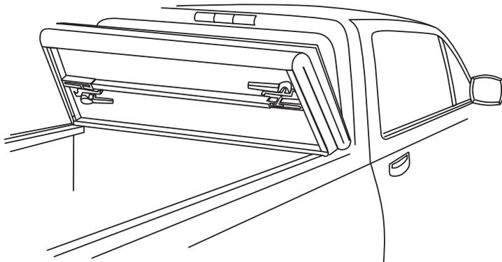
1. Position tonneau cover onto the top of the pickup box. See Figure 1.
