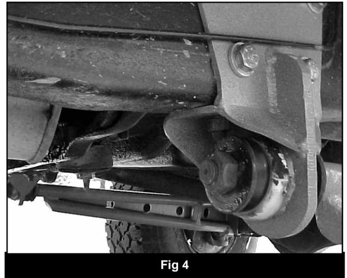
10. Raise bracket into position on the frame and secure with the 1/2" fasteners.
