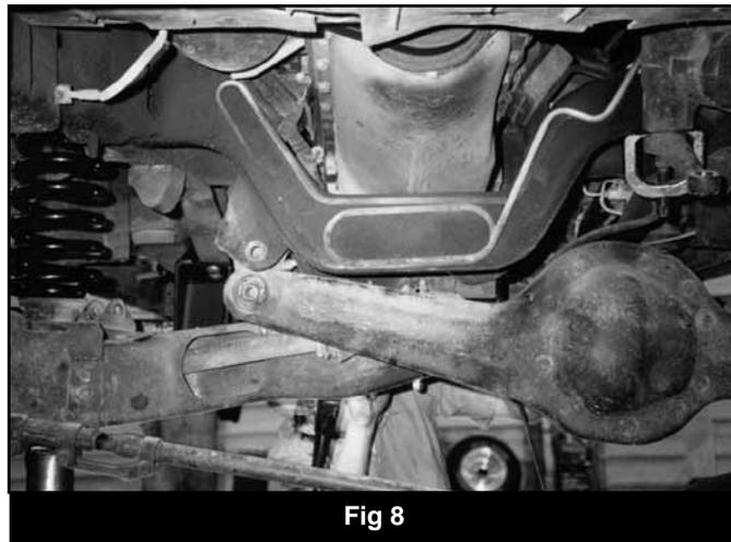
13. Remove driver side axle pivot bracket (located on passenger side). Install the larger BDS axle pivot bracket and attach using OEM fasteners and secure to OEM Specification. Attach the axle to the BDS bracket using the OEM fasteners in the hole appropriate of the coil spring being used. Tighten, but do not torque to specification at this time.
