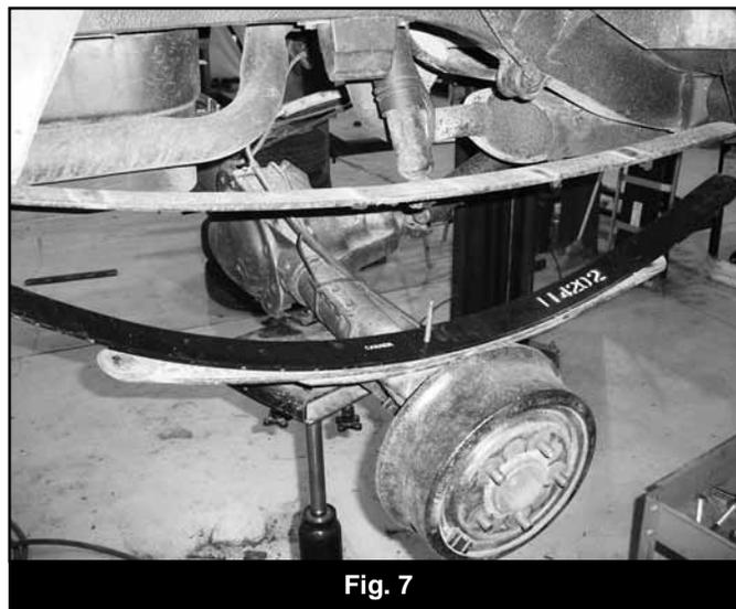
41. Using the C-clamps on each side of the center pin hole, compress the leafs together while aligning the new center pin through all of leaf center pin holes (from the bottom up). With the pack completely compressed together with the
