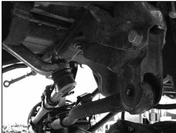
10. Vehicles WITHOUT transfer case indexing ring kit installed or gas model trucks: Disconnect the driveshaft from the front axle. Note: It may be necessary to heat the front axle yoke to get the loc-tite to break free. Retain all hardware. (Fig 5) (Diesel trucks w/ indexing ring kit installed may skip this step)
