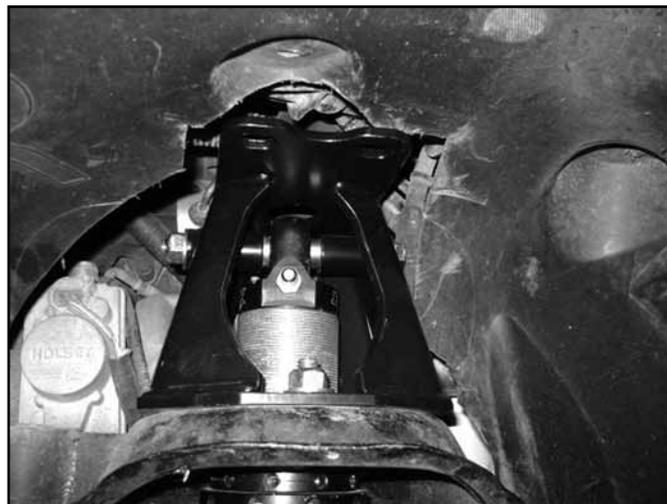
23. Attach the reservoir mount to the upper coilover mount with ½" hardware with washers and loc nuts. Tighten to 65 ft-lbs. Attach reservoir to the mount with hose clamps included with Fox Coilover Box Kit. (Fig 10a, 10b)
