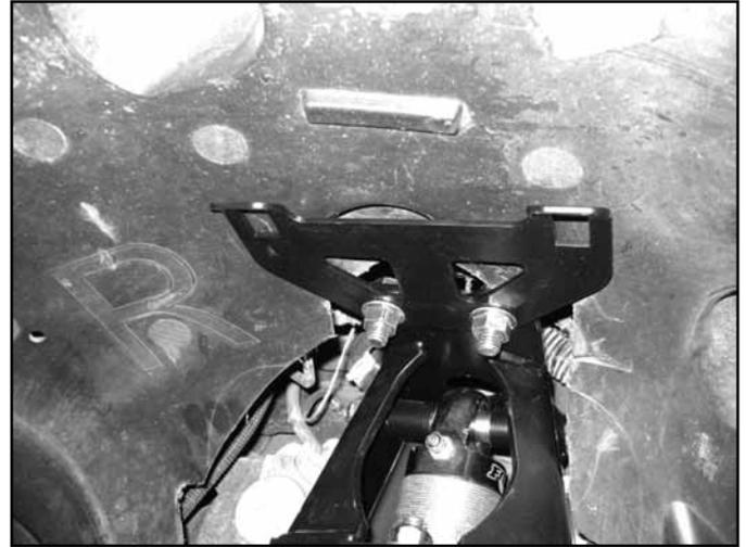
24. Allow the axle to droop out fully, reattach the driveshaft with factory hardware with loctite, tighten to factory specifications. If axle is unable to be reattached it may be necessary to clearance the dual cardan at the transfer case to allow for extra droop, additionally an indexing ring kit may be required as indicated in the pre-installation notes. Gas models may require exhaust modification at this time for driveshaft clearance at full droop.
