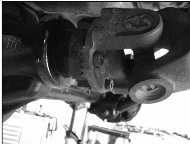
11. Disconnect the front shocks and allow the axle to droop out. Remove the coil springs, remove the front shocks. Check for adequate clearance of brake lines, ABS wires, driveshaft to exhaust (gas models), etc.
