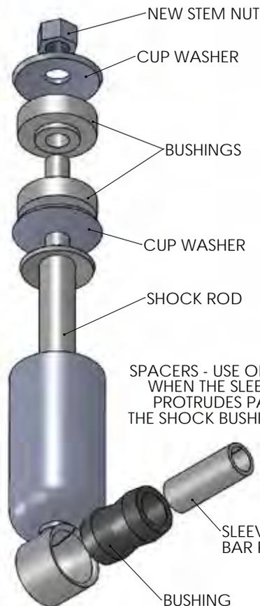
5500 AND NX<sup>2</sup> SERIES SHOCKS MUST BE MOUNTED WITH THE BODY FACING DOWN.
