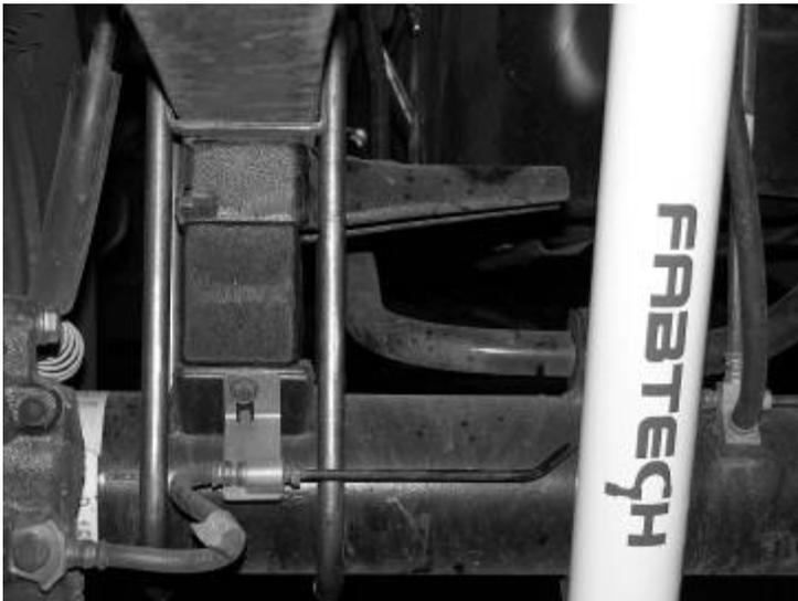
3. Install Fabtech shock part number FTS7266 Performance Shocks or FTS81005 Dirt Logic (not included) with the factory hardware and torque bolts to 65lbs.
