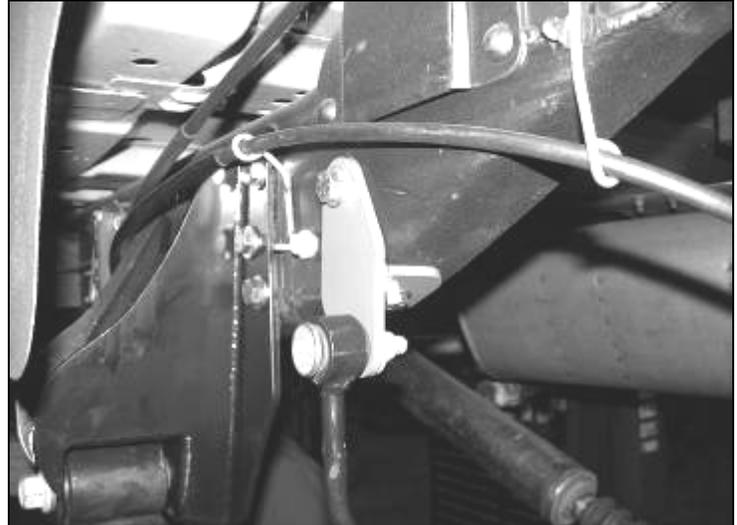
8. Install Fabtech shock part number FTS7266 (not included) with the factory hardware and torque bolts to 65 ft-lbs.
