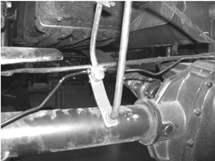
7. Locate the FT30240BK (driver) and FT30241BK (pass) Rear Sway Bar Drop Brackets. Remove the factory sway bar end links from the frame and save the hardware. Place the drop bracket onto the frame so that the hole in the new bracket is
