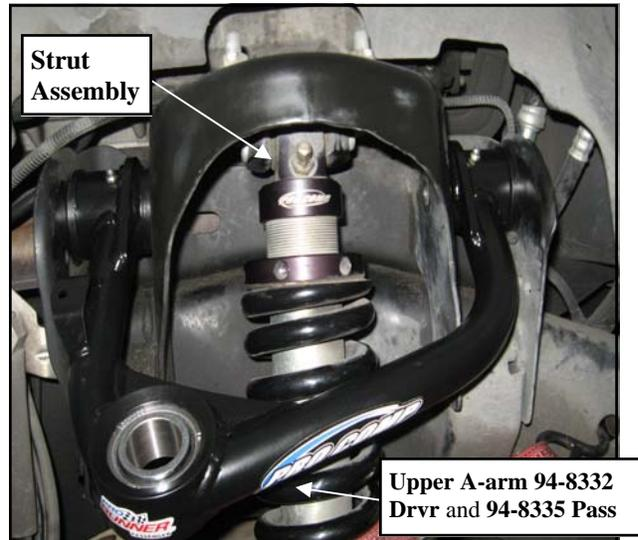
25. Insert spacer (90-4611 top and 90-4610 bottom) into the uniball on the Pro Comp upper A-arm.
