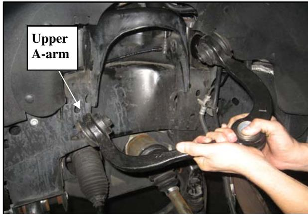
19. Install the (4 per arm) bushings (15-11329) into the Pro Comp upper A-arm (94-8332 Drvr and 94-8335 Pass).
