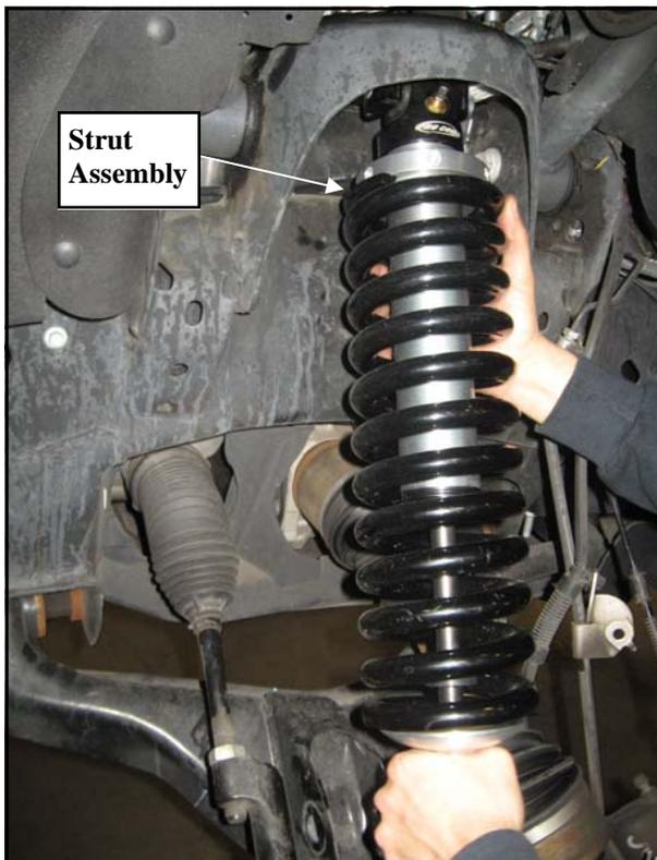
23. Install the supplied misalignment spacers and OE lower strut bolt in the original position that it was removed.
