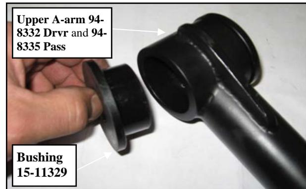
20. Insert the sleeve (90-8336) into the upper A-arm bushings.
