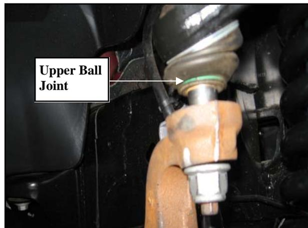
12. Remove upper ball joint nut to free the axle.
