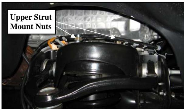
16. Remove the strut assembly from the vehicle.
