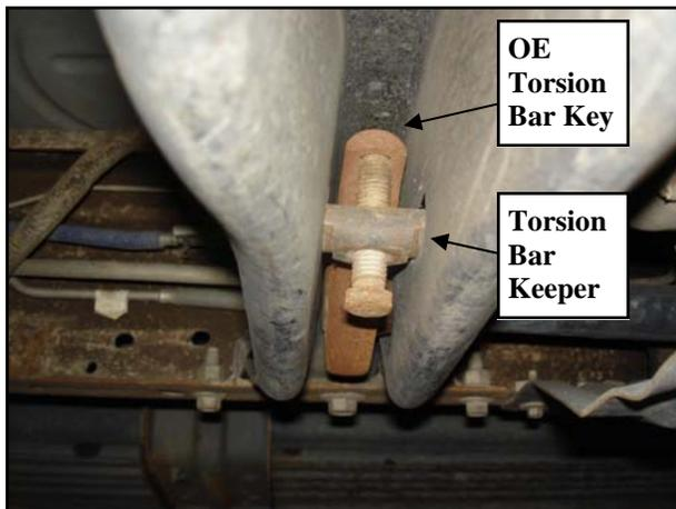
5. Starting on the driver's side, remove the torsion bar adjusting screw. Apply a small amount of lubrication grease to the torsion bar puller (67971 is recommended), threads and the puller shaft-to-adjuster arm contact point. Load the puller and tor-
