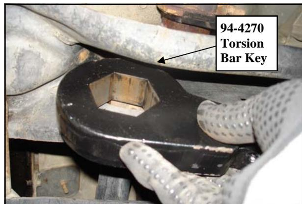
**IMPORTANT! Make sure Torsion Bar is extended at least 1/4" inch through the Torsion Key.**
