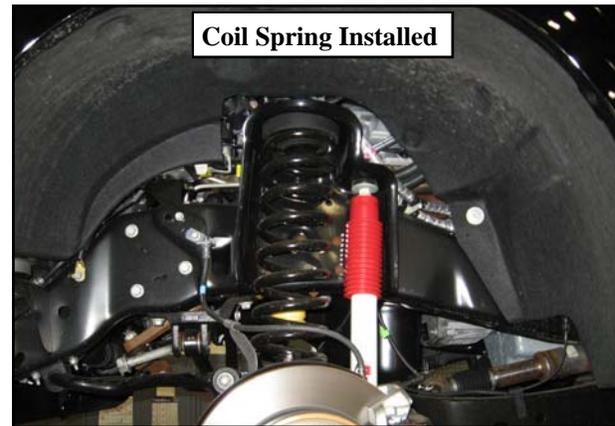
13. Now would also be a good time to inspect the front shocks for damage or fluid leakage. Replace if necessary.
