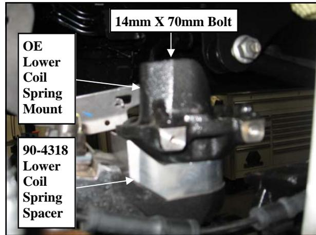
12. Compress the spring down, install the OE isolator and reinstall the spring. Be sure to line up the previously applied coil spring reference mark.
