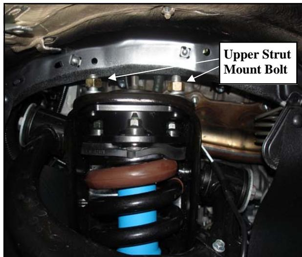
8. Remove the strut assembly from the vehicle and install securely in a bench vise.
