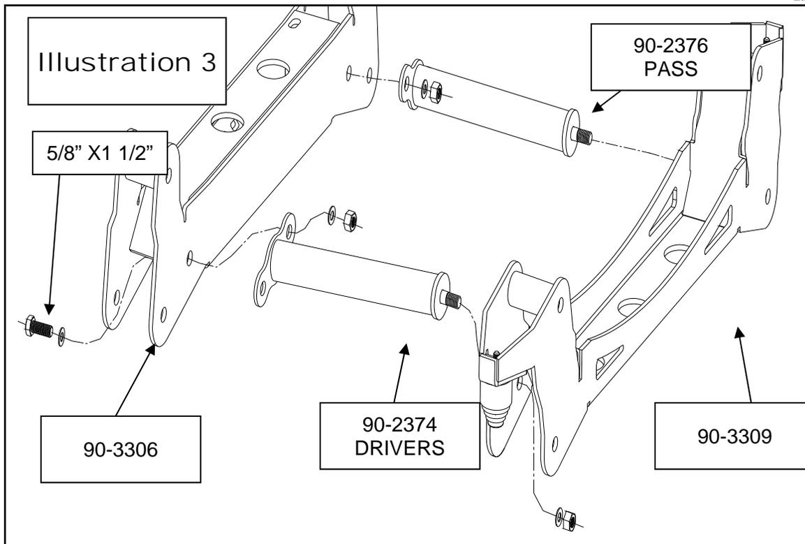
26. Place the rear cross-member, **90-3309**, into the existing lower control arm mounting position using the **OEM** hardware previously removed. Make sure that the bolt heads are facing to the rear of the vehicle. Do not fasten at this time. **SEE ILLUSTRATION 2.**
