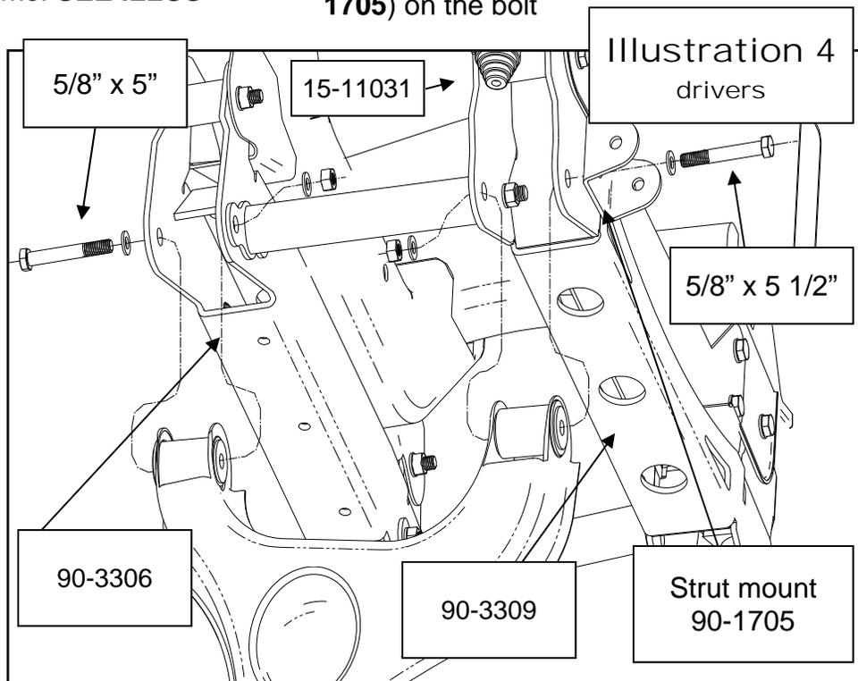
then install the bolt to the rear of the lower control arm. Use **5/8" X 5.5"** hardware provided from pack **90-6227**. Make sure that the rear bolts heads are facing to the rear of the vehicle. Make sure that the front bolts heads are facing to the front of the vehicle. Do not torque at this time. **SEE ILLUSTRATION 2.**
