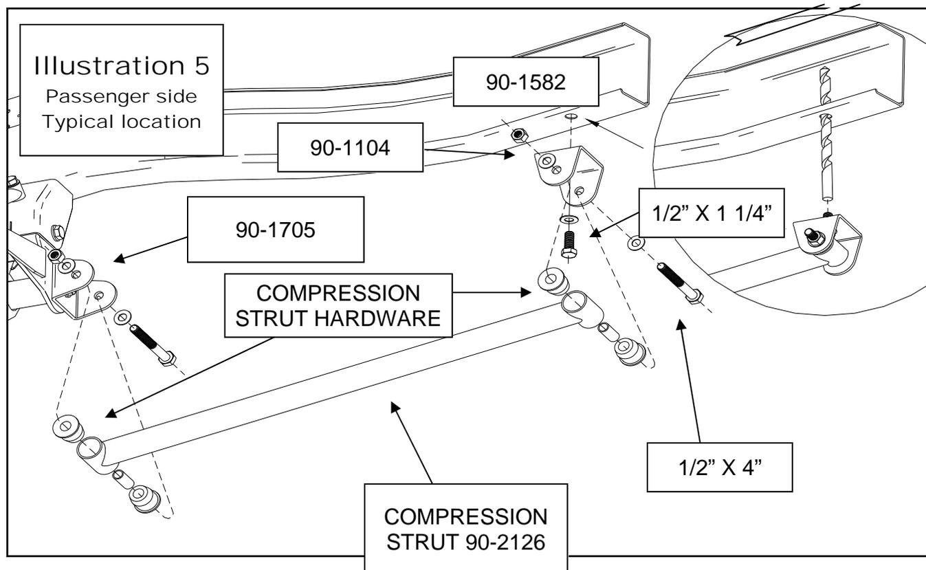
pression struts using the supplied 1/2" X 4" hardware.
