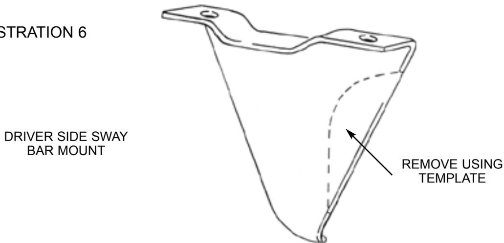
ILLUSTRATION 6. Remove the crossmembers from the anti-sway bar and trim using a saber saw or die grinder. File any sharp edges and reinstall crossmembers.
