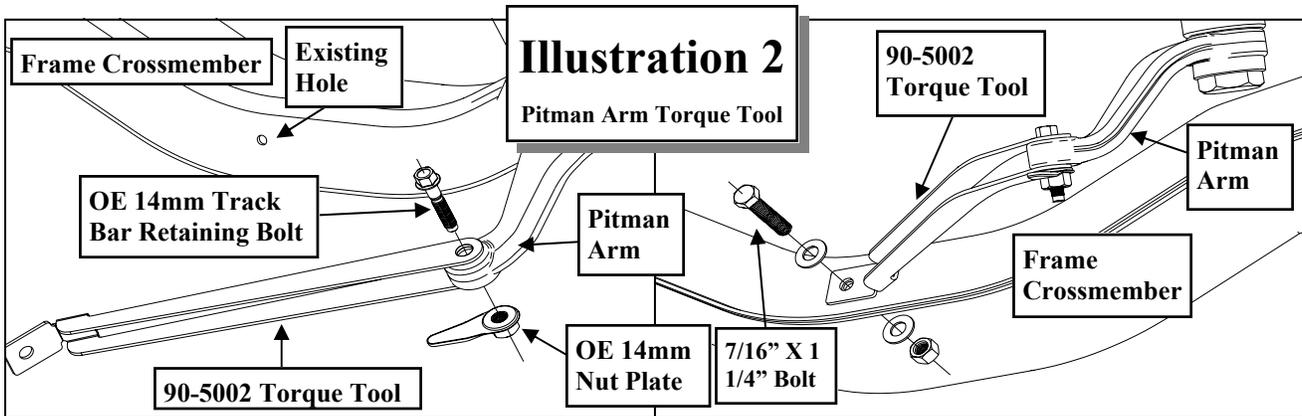
using the supplied 7/16" X 1 1/4" bolt and hardware. See Illustration 2.
