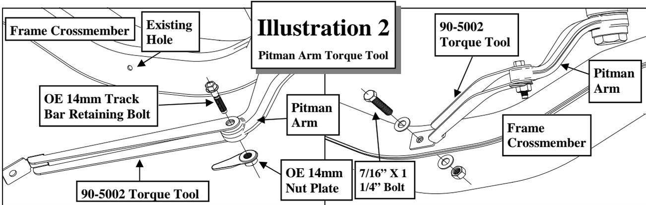
to be turned in order for the hole in the torque tool and the frame crossmember to line up. Once the bolts are tightened the torque tool will align it's self properly.
