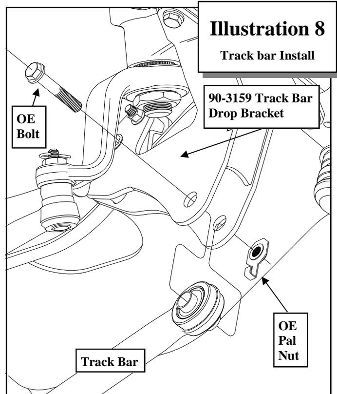
**NOTE:** You may find that having someone inside the vehicle and moving the steering wheel from side to side will aid in the alignment of the track rod. **DO NOT** start the engine for this! You only have to move it enough to line the holes up on the track bar mount.
