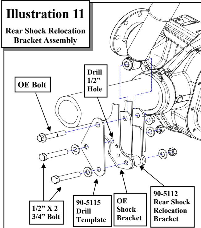
17. Make sure the bracket is rotated fully into place until the welded portion of the bracket (**90-5112**) inside **OE** axle bracket and using the hole in the drill template as a guide mark the axle bracket for drilling. See ILLUSTRATION 11.
