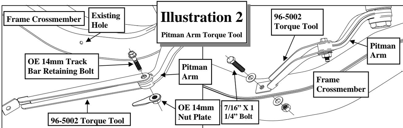
*shaft. If you do not have this tool, a length of chain or a flat bar with two holes is a suitable replacement.*
