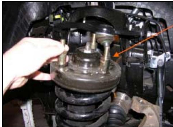
9. Apply the thread lock to the (3) strut studs and install the stud extenders and tighten down.
