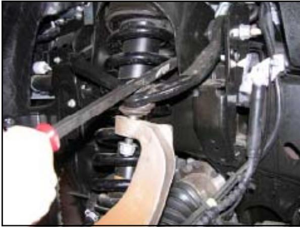
strut studs will go through the strut tower, use the new lock nuts and washers to install the strut.
