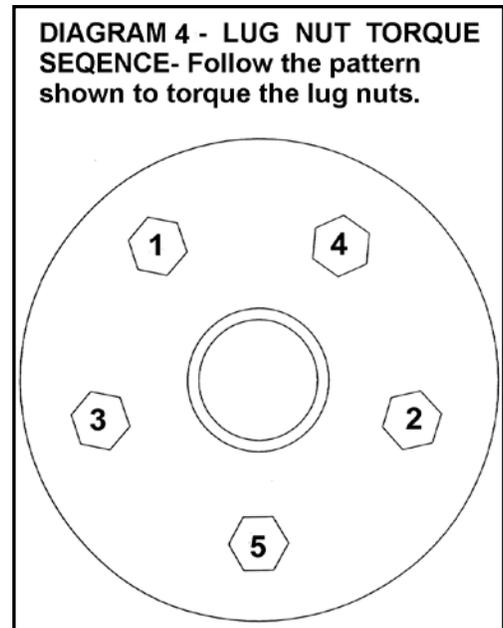
**16) TIGHTEN the SUSPENSION COMPONENTS...**
