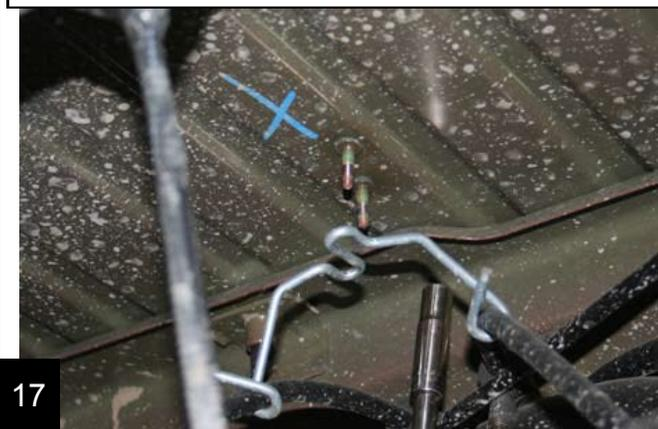
Remove the brake line mount from the frame with a 10mm.
