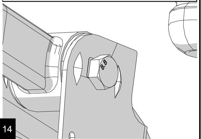
Remove the shock at the axle with an 18mm. (See 999207 Shocks/Rear/Removal)
