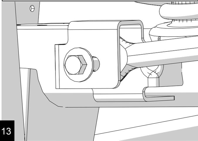
With a 21mm loosen all rear control arm bolts. DO NOT REMOVE ARMS OR BOLTS.
