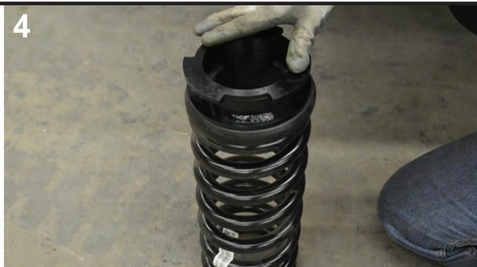
Re-install the isolator onto the spring, and mount the Traxda Coil Spacer above it. Repeat steps 3 and 4 for other side of vehicle.
