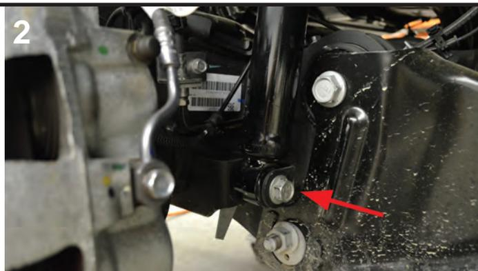
Disconnect the front shock absorbers at the axle mounts on both sides. Carefully lower the front axle using jack until the coil spring is loose.
