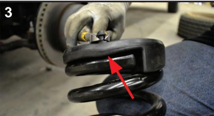
Remove the coil spring and rubber spring isolator from the vehicle. Cut the nipple off of the rubber spring isolator.
