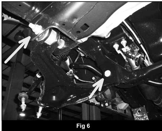
16. Mark the struts to distinguish between driver's and passenger's. In addition, mark the relationship between the coil and the lower strut mounting hole and finally the top plate and the rubber coil seat.
