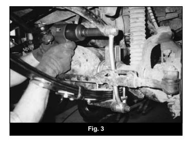
15. Bounce the front of the vehicle to settle the suspension. Torque the u-bolts to 70-85 ft.lbs. Torque the 9/16" hanger bolts to 95 ft.lbs. and the 1/2" shackle bolts to 65 ft.lbs. Attach the track bar to the track bar relocation bracket with a 12mm x 70mm bolt, nut and 7/16" USS washers from bolt pack #904. Turn the steering wheel to help align the holes. If necessary the track bar can be loosened at the frame to provide extra movement. Torque track bar bolts to 55 ft. lbs.
