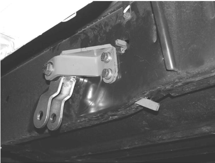
5. Locate the Fabtech traction bar FT90052BK. With the Heim Joints installed connect the traction bar to the rear axle bracket with the supplied 3/4" x 2 1/2" bolts, washers, and c-lock nuts. Leave loose. When attaching the traction bar to the axle make sure the heims are straight up and down.
