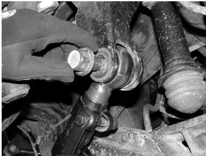
7. Center the axle accordingly using the adjuster sleeve on the track bar. After all adjustments have been made lock down the adjuster sleeve with the cross bolts. It is important that the sleeve is locked down with cross bolts perpendicular to the diff cover. **SEE PHOTO BELOW**
