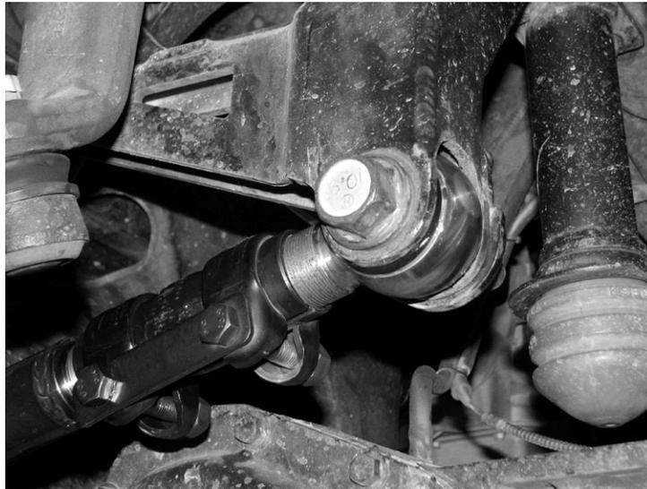
8. After the track bar is installed it may be necessary to have vehicle Alignment performed
