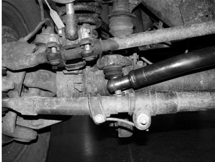
6. Install the bushing end of the track bar into the drop bracket on the frame. Tighten to 406 ft-lbs. **SEE PHOTO BELOW**
