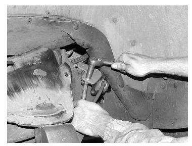
3. Attach the brake line relocation tab to the top of the frame rail using the original bolt, only hand tighten. Using the supplied 1/4" bolt, flat washers and lock nut, attach the brake line to the relocating tab. You may have to slightly bend the factory hard line. MAKE ONLY SLIGHT BENDS, DO NOT KINK THE BRAKE LINE.
