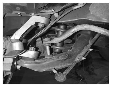
12. Slide the ABS sensor wire behind the steering arm. Route the wire along the rubber brake line and place it back in the retaining clip on the upper ball joint. Using the supplied cable ties, attach the wire to the brake line. Tighten the retaining clip on the upper ball joint, do not crimp the wire.
