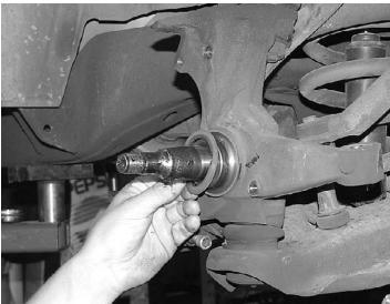
6. Remove the three bolts securing the dust shield to the spindle and set the shield aside. Remove the rubber ring from the spindle and set this aside with the dust shield, they will be reinstalled later.
