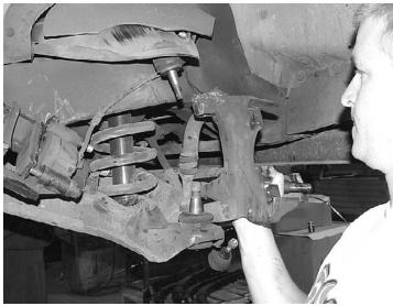
7. If you do not have the factory shock still installed on the truck, support the lower control arm (LCA) with a floor jack. Remove the cotter pins from the upper and lower ball joints. Remove the castle nuts securing the upper and lower ball joints to the spindle. Use a ball joint puller to separate the spindle from the ball joints and set the spindle assembly aside.
