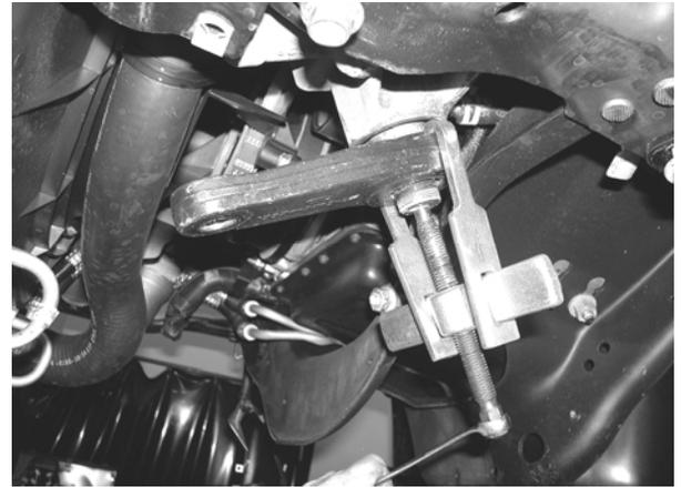
9. Locate FTS30122 new drop pitman arm. Attach to the steering box in the same indexed position as the factory pitman arm was when removed. **Install the provided FT30258 Sector Shaft Nut and torque to 350 ft. lbs. (Note: this is a one-time only use nut, once it is tightened on the sector shaft and removed, it must be discarded.**
