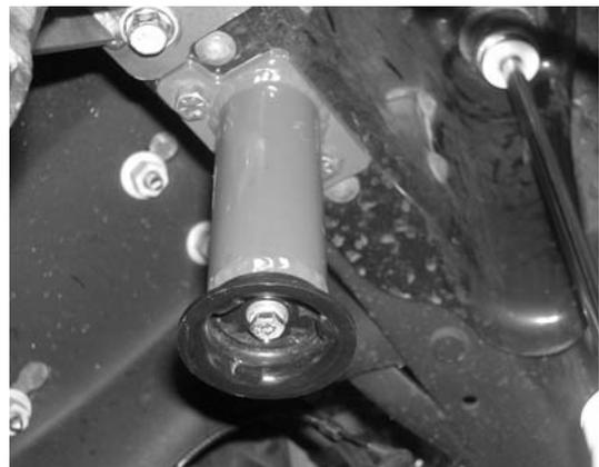
Photo shown without bump stop installed
