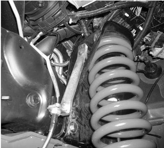
22. Reattach the ABS line to the radius arms in the original location using the original hardware. Plug the ABS line back together at the fender well.
