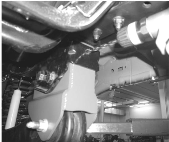
15. Reinstall the radius arm onto the truck using the original hardware. Attach to the axle first then to the new drop bracket using the rearward hole. Leave loose at this time. SEE DRAWING IN NEXT COLUMN.
