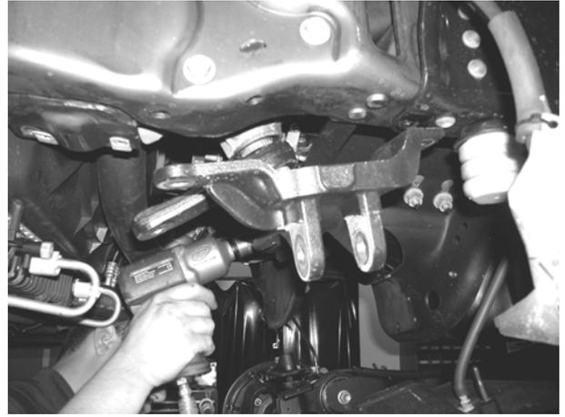
8. Remove the factory pitman arm from the steering box using a large pitman arm puller or large two-jaw puller. Save the hardware and discard the pitman arm. SEE PHOTO BELOW.
