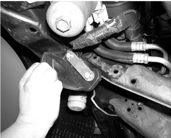
6. Remove the drag link from the pitman arm and save factory hardware. You will need to strike the pitman arm with a large hammer to dislodge the drag link for the pitman arm. **USE CARE NOT TO KIT THE THREADS ON THE DRAG LINK!**
