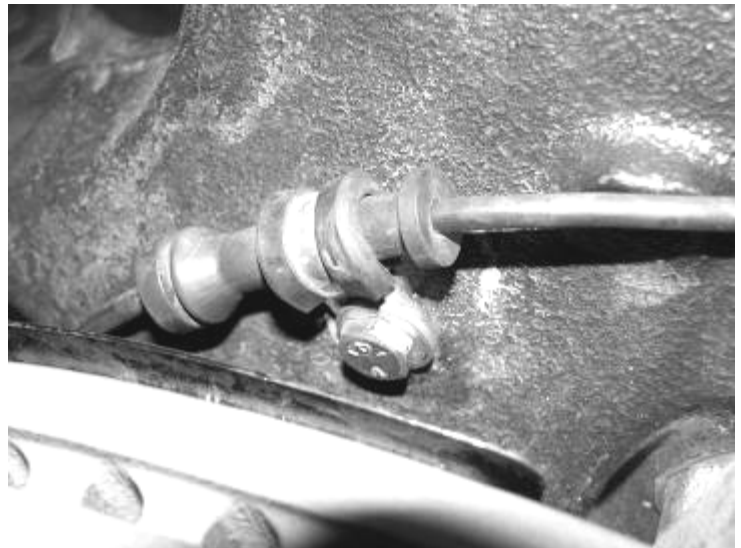
Photo shows Adel clamp attaching ABS Line to knuckle
