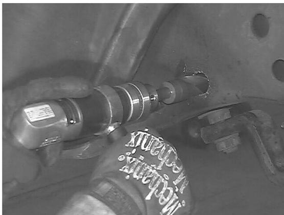
4. Place the upper shock mount back onto the coil tower. Slide the driver's side frame sleeve (2 13/16" long) into the new 1" hole. Place a 1/2" x 4" bolt through the front tube of the upper shock mount, into the frame sleeve and through the back of the frame. Use a 1/2" flat washer and lock nut
