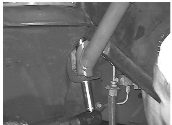
6. Position the lower shock mount below the lower coil spring mount. Secure the bracket to the lower coil spring mount using the supplied  $\frac{1}{2}$ " x  $1\frac{1}{2}$ " bolts,  $\frac{1}{2}$ " flat washers and  $\frac{1}{2}$ " lock nut. You will need to drill out the 2 factory holes to  $\frac{1}{2}$ ". The rear hole will use the  $\frac{1}{2}$ " x  $4\frac{1}{2}$ " bolt, nut and washer, throw the existing link arm hole. SEE PHOTO BELOW. ( PICTURE IS OF PASSENGER SIDE )
