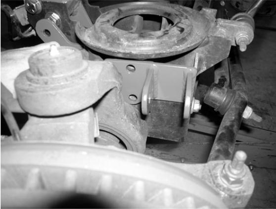
7. Repeat steps two through six on the passenger's side of the truck. The passenger's side of the truck will use the  $\frac{1}{2}$ " x  $3\frac{1}{2}$ " bolt and  $1\frac{7}{8}$ " frame sleeve on the front tube of the upper shock mount.
