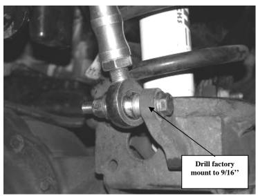
19. Locate the supplied ½" button head bolts and the sway bar bushing along with the cup washers. Attach the bushing end of the sway bar end links to the sway bar, leave loose at this time. At times this may be easier to attach when the truck is completed and on the ground. SEE PHOTO ON NEXT PAGE
