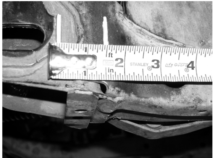
Measure 1 1/2" inward from the cam pocket For cutting on both sides
