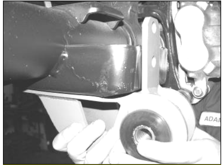
photo shows bracket with proper clearance on diff bracket paint all exposed / raw areas after all cutting and grinding is done
